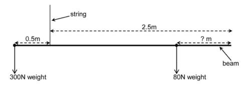
How far from the other end must a weight of 80N be placed for the beam to be balanced?
